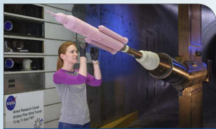
Amber Favaregh of NASA's Langley Research Center prepares a model of the Space Launch System rocket for testing with pressure-sensitive paint in a wind tunnel at NASA's Ames Research Center. Credit: NASA/Dominic Hart
