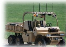
GUSV (Optionally Autonomous ITV)
